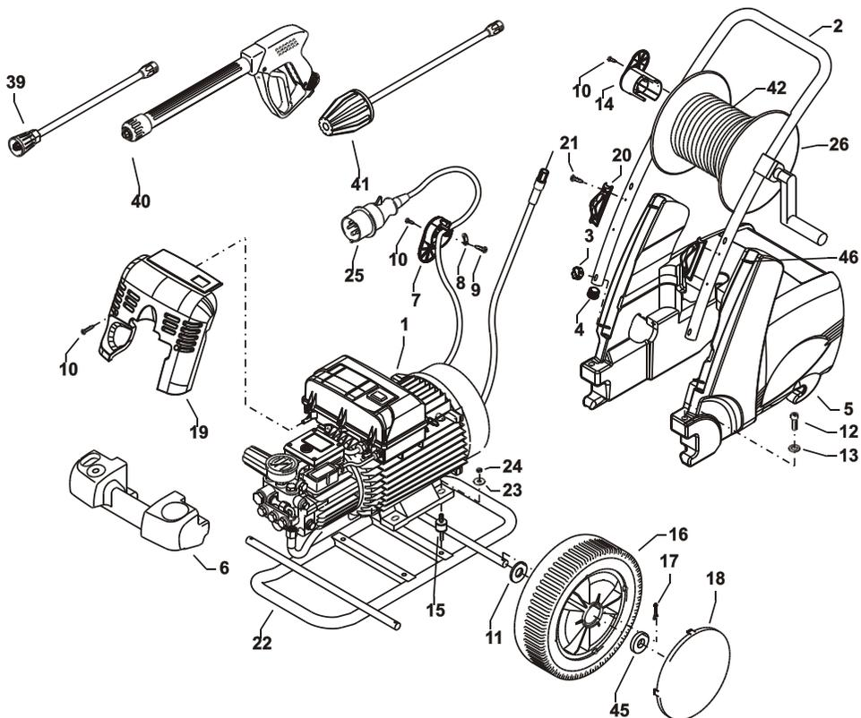
**Komplettaggregat quadro 1500 TS / TST**
