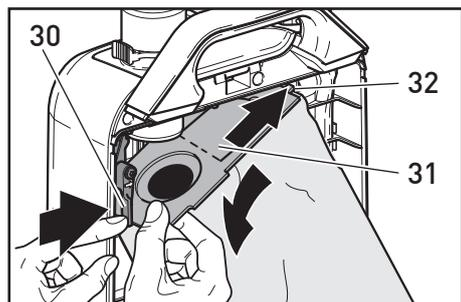
To fit a new dust bag, Slide the right side of the bag top (32) into the holder and fit the dust inlet of the bag top over connecting tube until the filter bag latches into the lever (30).
