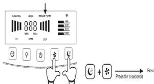
We recommend you to replace H.E.P.A filter H14 when REPLACE FILTER message is displayed on the screen. After replacing H.E.P.A filter, please proceed as follows:
