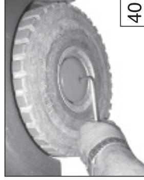
Control monthly wheel bolt for tightness. (picture 40)
