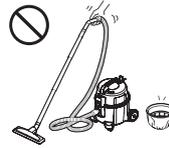
Be sure to replace the filter after disposing of the dust. If the cleaner is used without replacing its filter, dust will be sucked directly into the mechanical parts and may damage the motor.
