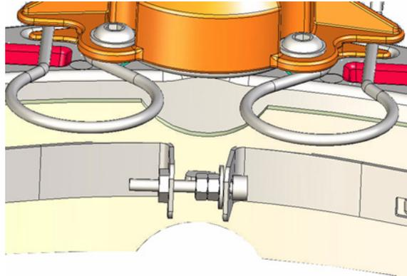
Picture 13: Front blade fixation
