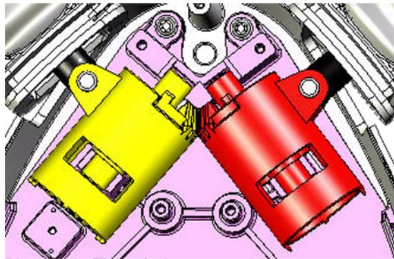
Picture 4: Throttle levers position
