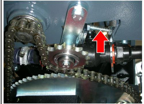
6. Verify the steering axle clearance. If necessary screw the **bush**. Verify the complete an correct movement.
