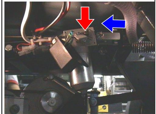
5. Check, with the brush assembly completely down of the machine, the wheel touches but is not blocked against **lateral blade**.
