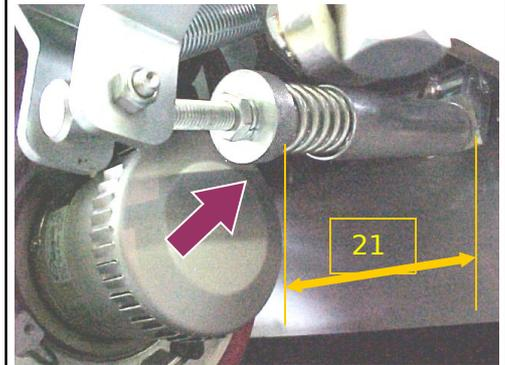
3. Adjust the brush assembly inclination: if necessary (so if you have a different current consumption on the two motors) and adjust the inclination operating on the **eccentric bushers** that block the lower right and left arms:
