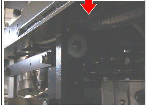
4. Adjust the **microswitches** of the side movement of the brush base which are on the actuator. The more distant to the actuator has to switch when the wheel touch the end stroke blade. Regulate the nearest one to have a **distance** between the wheel and the end stroke blade of about:
