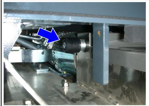
3. adjust the position of the second **microswitch** to stop the lowering when the most high edge of the arm is at **470mm** from the floor.
