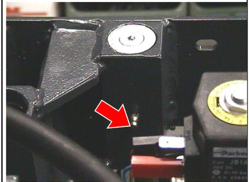
4. Verify the cleanness and functionality of the carbon brush cover of the **brush motor**.
