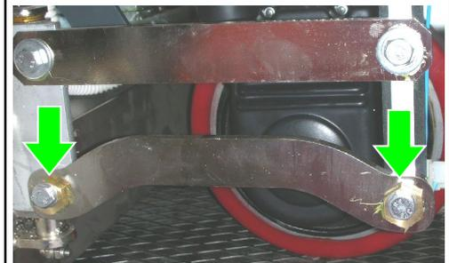
2. verify that the brush base can move free (about 100mm) to the center of the machine in case of incident.
