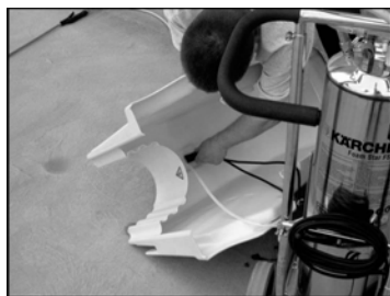
Check hose and switch connection.
