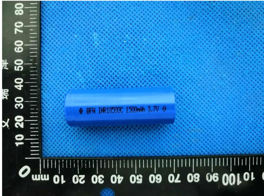
Figure 11 Front view of cell (18500 1500mAh)
