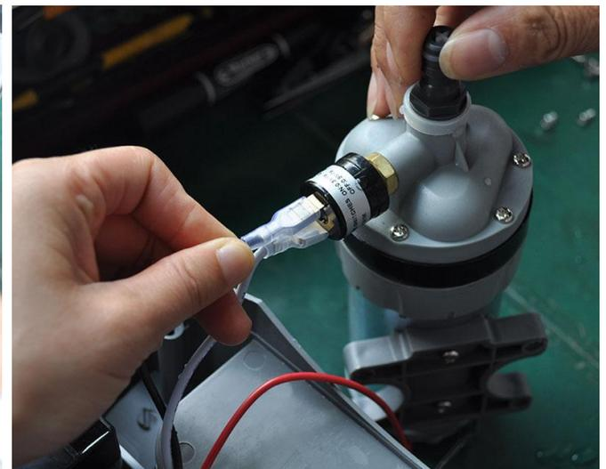
To take out the pump from the housing, disconnect the wire from pressure switch
