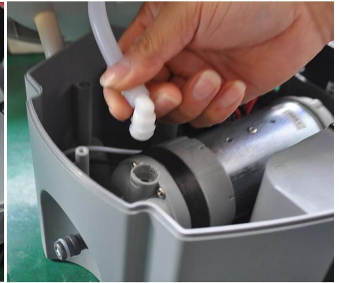
After open the upper cover, twist off the hose which is connected the pump
