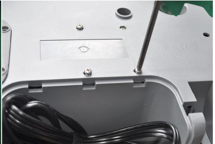
Unscrew the four screws on the bottom to release the pump from the housing
