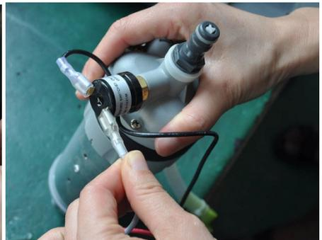
Disconnect the wire on pressure switch
