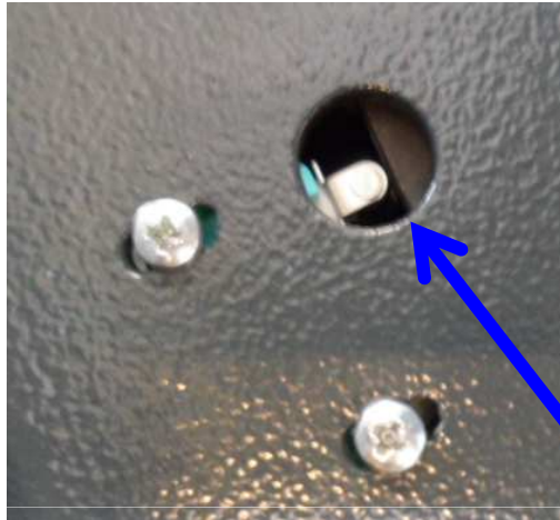
Micro switch for automatic reduction of speed on bends
