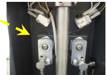
Micro switches for vacuum and brushes motor
