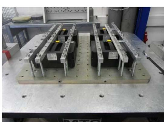
Shock machine with test samples (top view)
