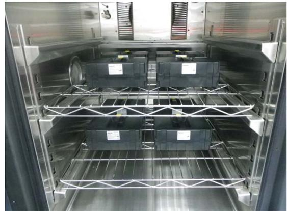
Batteries inside temperature chamber
