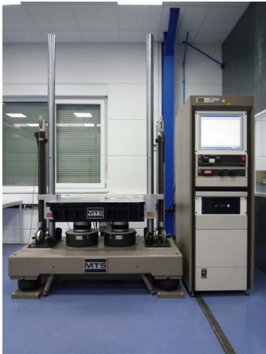
38.3.4.4 Set-up of test 4: Shock
