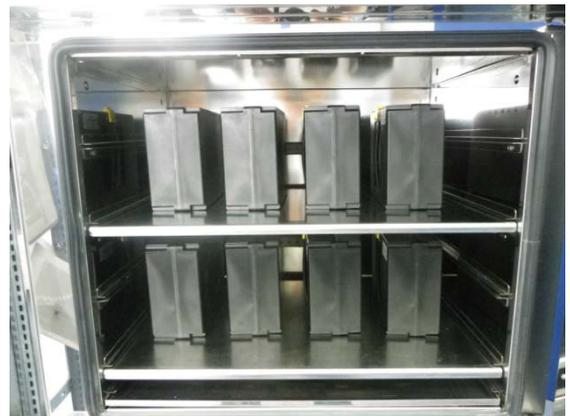
Batteries inside altitude chamber
