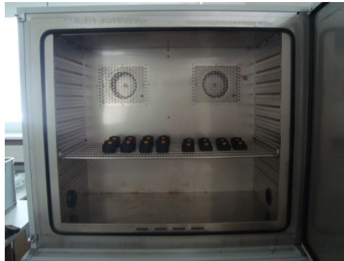
Figure 3: Thermal test in climate cabinet with the batteries inside
