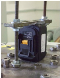
Figure 7: Shock test on shaker table with the batteries
