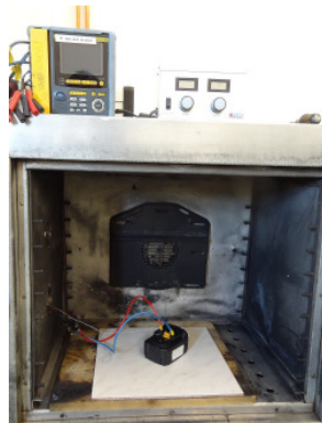
Figure 11: Overcharge test in safety cabinet with charge equipment (overcharge current 6 A, overcharge voltage 25.0 V)
