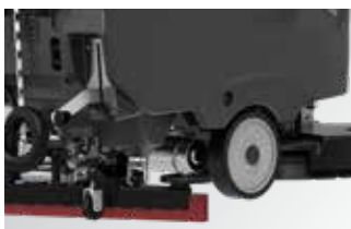
Front-wheel drive equipped with reverse
