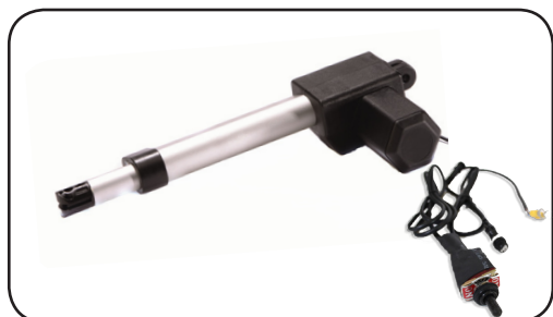
EAN: 5710122120627 Dimension : 400x220x80 mm Engine: 12 V electric (24 V) Force: 300-400 kg Speed: 8 mm/sec Build in length: 325 mm Shoot length: 150 mm Spare parts: See pricelist
